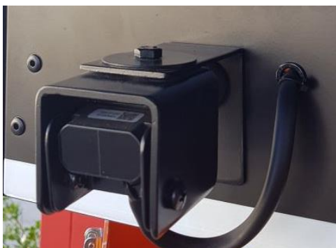
Vehicle Detection LiDAR Unit fitted at bottom of eSTOP™ Unit, facing the traffic. Will detect objects up to 4 meters in front of unit.
