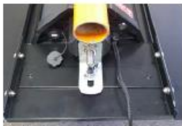
5. Insert bolt then tighten wing nut.
