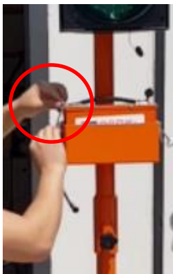
Lock latches to secure battery box
