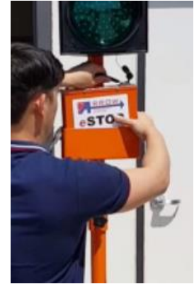
Insert battery pack into battery holder
