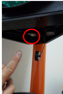
Switch on lantern
