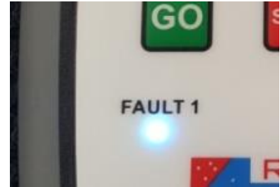
Indicates in Cyan colour when 2 units are paired to one GO button.
