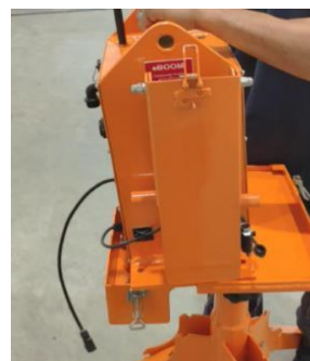
Slide the eBOOM™ body onto the tray.
