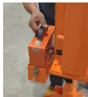
Insert Battery pack into the Battery holder.
