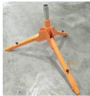
Adjust each leg so that the tripod stands stable on the ground.
