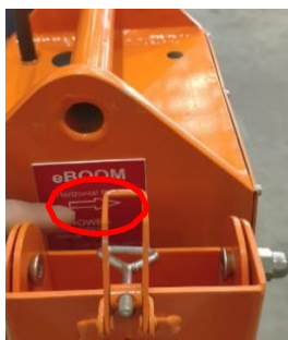
Maintain the same orientation as shown. The arrow sign indicates the direction of the boom arm movement in horizontal position.
