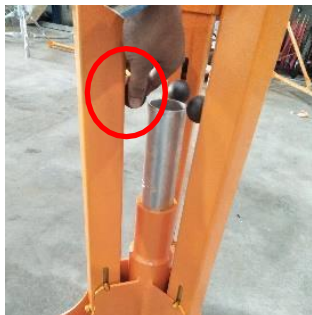
Pull the pin upwards to release the leg
