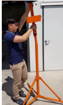
Slide lantern into the center locking column
