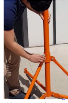
Slide pole up and down to adjust height then release pin to lock in place
