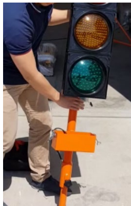
Check antenna is vertical. Use two hands to lift traffic lantern onto base
