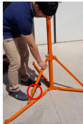
Place legs onto a flat surface and align adjustable locking column with pin holes for uneven surface. (red circle)
