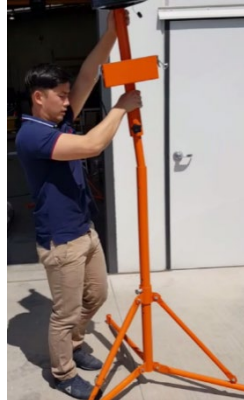
Slide lantern into the center locking column
