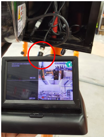
Figure 3. DVR output and LCD
