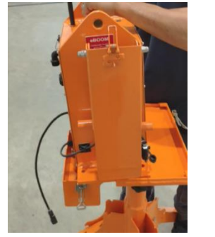
Slide the eBOOM™ body onto the tray.
