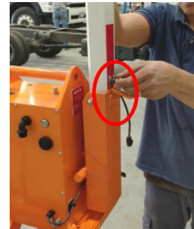
Lock latches to secure the arm
