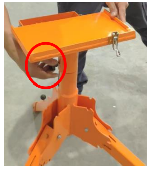
Secure the tray using locking screw.
