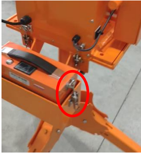
Lock latches on both sides to secure the battery in place.
