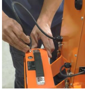
Connect the Power cable. Connector latches once positioned in place.
