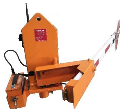
eBOOM™ arm dislodged due to motorist crashing into the arm.
