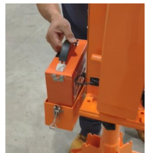
Insert Battery pack into the Battery holder.
