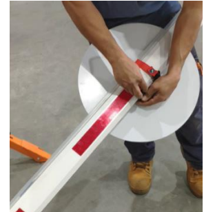
Secure the STOP sign using the lockable latches.
