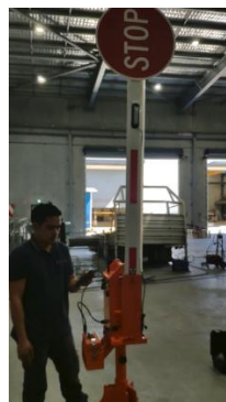
Ensure the orientation of the arm is such that the STOP sign faces the incoming motorists
