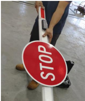
Extend the eBOOM™ arm to required length. Most instances this is 3m.
