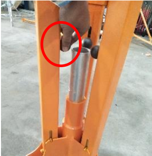
Pull the pin upwards to release the leg
