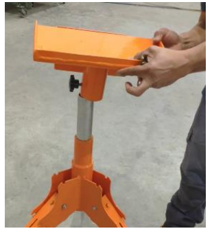
Insert the eBOOM™ tray to the centre column.
