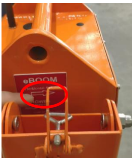
Maintain the same orientation as shown. The arrow sign indicates the direction of the boom arm movement in horizontal position.
