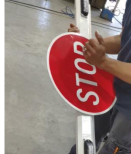
Attach the STOP sign to the eBOOM™ arm. Note this may not be required in certain States and applications.
