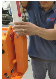
Insert the eBOOM™ arm into the eBOOM™ arm holder.
