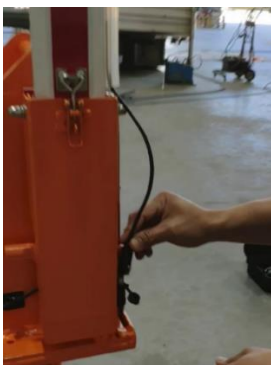
Attach the eBOOM™ arm cable to the eBOOM™ as shown.
