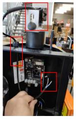
b. Once the cable is through the gland and is inside the lantern housing, connect the cable and terminal into the connector shown below. You should be able to feel a small click once is properly inserted, try pull the cable to double check if it is in properly. Brown wire connects to the top left slot and blue wire connects to bottom right slot shown below.
