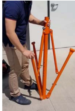
Extend legs out by pushing towards the ground
