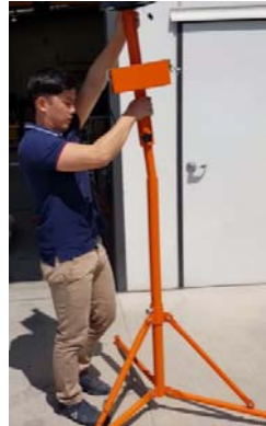
Slide lantern into the center locking column
