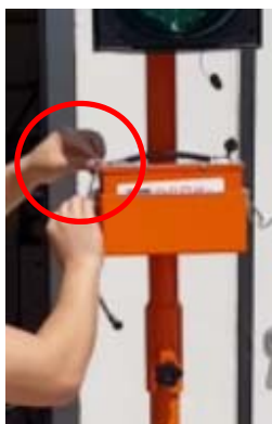
Lock latches to secure battery box
