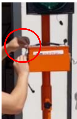
Lock latches to secure battery box
