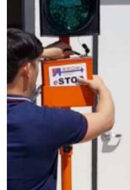
Insert battery pack into battery holder
