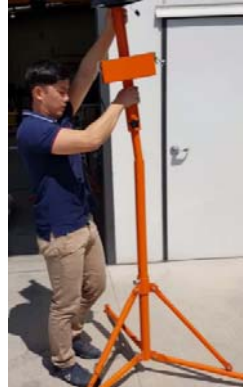
Slide lantern into the center locking column
