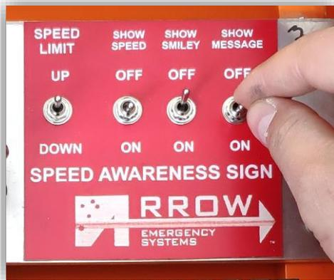
**SHOW SPEED** – If the show speed is switched on. The unit will display the detected vehicle speed for 2 seconds. The color of the LED display will be green if the drive is below the limit, and red if the drive is over the limit.
