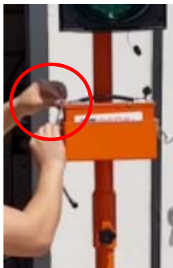
Lock latches to secure battery box
