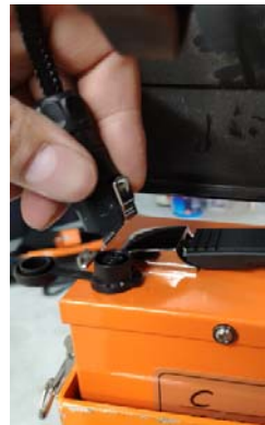
Connect power cable. Connector latches once pushed in place.
