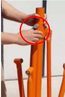
Pull spring pin to release leg
