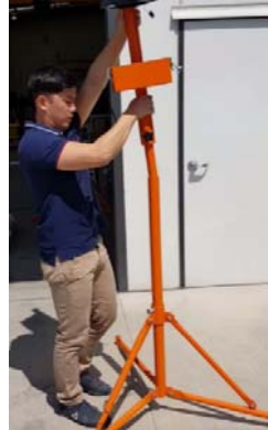
Slide lantern into the center locking column
