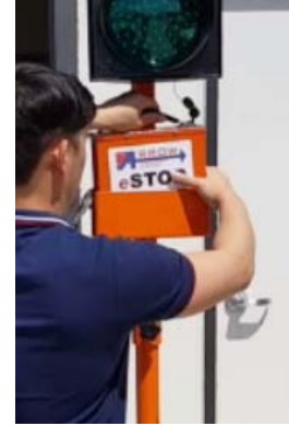
Insert battery pack into battery holder
