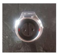
6. After installing the new connector, before putting the lid cover back on, be sure to silicon around the connector screw and around the lip of the cover highlighted in screen
