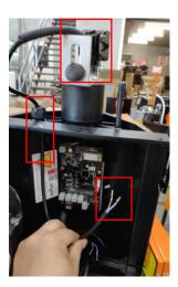
b. Once the cable is through the gland and is inside the lantern housing, connect the cable and terminal into the connector shown below. You should be able to feel a small click once is properly inserted, try pull the cable to double check if it is in properly. Brown wire connects to the top left slot and blue wire connects to bottom right slot shown below.
