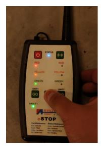
Battery level check using a HRC – once a lantern is paired and communicating with the HRC, the lantern battery level can be check by pressing the STOP button during test mode. Once it is pressed the green, yellow and red LED will light up representing a battery bar of 4 levels.
