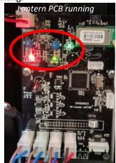
**Switch** - If the fuse is okay, the controller PCB LEDs are running and a known working battery is used but the switch LED is not on, then the switch is faulty.
