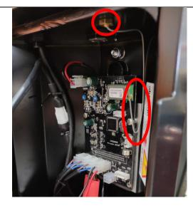
4. **Lantern aspects not lighting up** could be cause by a faulty lantern aspect or a faulty lantern controller PCB. During operation a red fault light indicates a faulty lantern aspect.
