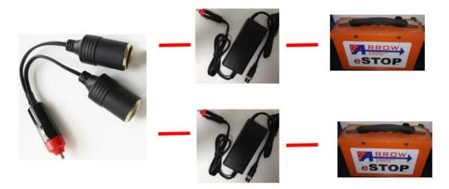
**Option 2**: Double cigarette socket where input connects directly to a battery with fuse holder, make sure fuse is 10A, battery is 12V.
