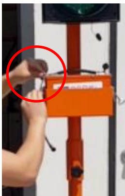
Lock latches to secure battery box
