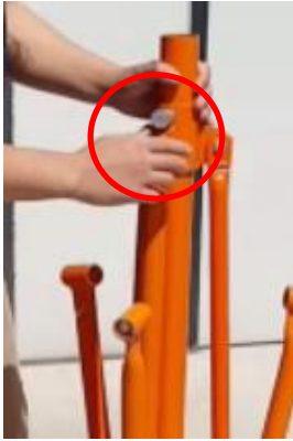
Pull spring pin to release leg
