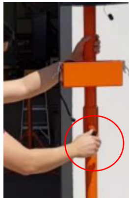
Secure with locking screw to stop lantern from rotating
