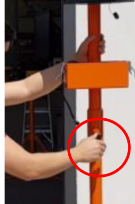
Secure with locking screw to stop lantern from rotating
