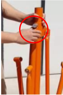
Pull spring pin to release leg
