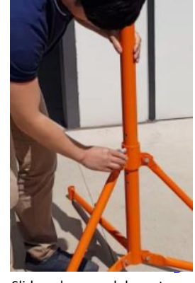
Slide pole up and down to adjust height then release pin to lock in place
