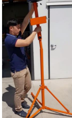
Slide lantern into the center locking column
