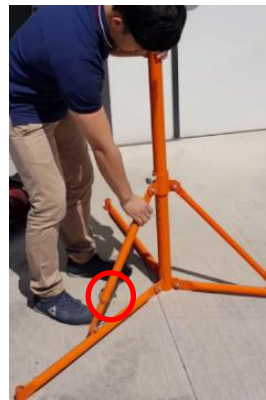
Place legs onto a flat surface and align adjustable locking column with pin holes to for uneven surface. (red circle)
