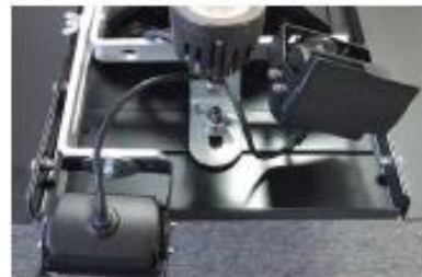
6. Adjust camera bracket and align hole on the top side of the target board, then tighten wing nut.
