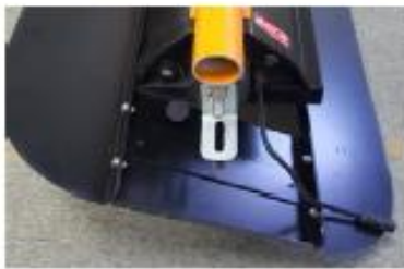
3. Lift one side of the target board over and behind the lantern edge.
