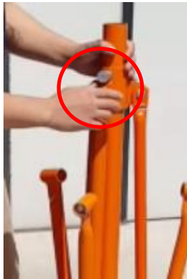
Pull spring pin to release leg
