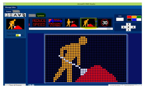
You can also edit the symbols by using the drawing tools, in this case the shovel is changed to amber color using the pen tool. Note: the background is black so to erase an area of the image,
